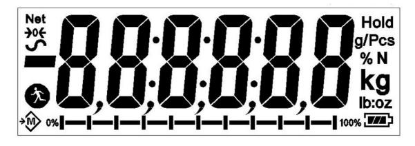
Other symbols will show when a weight has been tared (NET) the scale is at zero and stable, if a value has been stored in memory or when the animal weighing function has been enabled. A battery symbols will show the state of charge of the internal battery.
