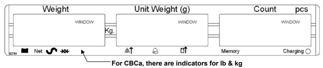
The scale will show the model No in the "Weight" display window (e.g. CBC 30- where 30 denotes the maximum capacity of the scale in Kg) and the current hardware and software revision numbers in the "Unit Weight" display window .Next a self-test is followed. At the end of the self-test, it will display "0" in all three displays, if the zero condition has been achieved.
